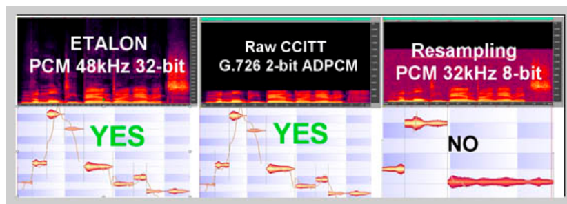
Fig. 3. Examples of immunity (YES) and non-immunity (NO) of the embedded data to modification in transmission environments.
