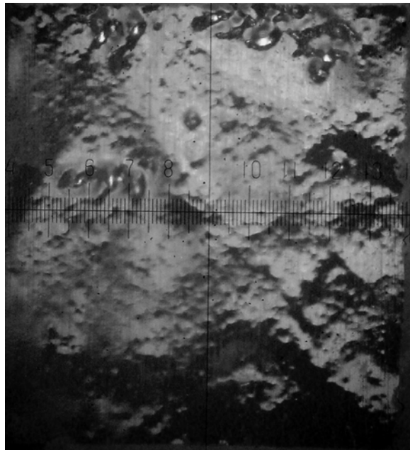
Fig. 2. An example for deformation situation of a foil by cavitation bubbles.
