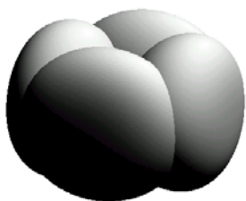
Fig. 3. Beam pattern of the infrasonic frequency detector
