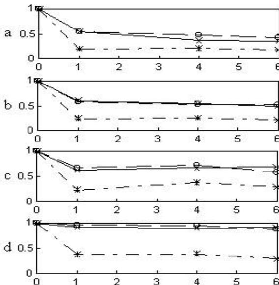
**Fig. 2.** Dependence of peak significances of the short temporal correlation function versus distance among hydrophones by different distances to source a — 304 km; b — 154 km; c — 56 km; d — 14 km.
