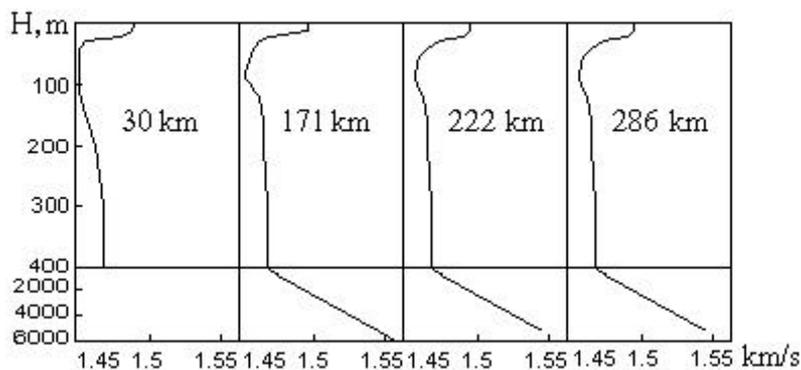
**Fig. 1.** Dependences of sound speed versus bound in the four dots of track (digits by curves — distance from hydrophones)
