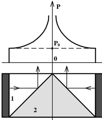
**Fig.1.** Antenna of pump and sound pressure distribution on it aperture.
