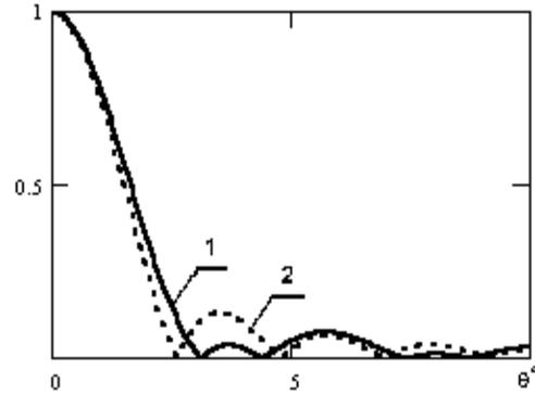
**Fig.2.** The directivity diagrams of: 1- the antenna, presented in Fig.1.; 2- the circular piston.
