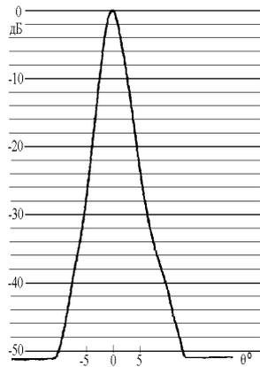
**Fig.5.** The parametric antenna directivity diagram, F=80 kHz.
