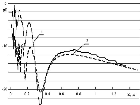
**Fig.4.** Axial distribution of sound pressure: 1- experimental; 2- theoretical.
