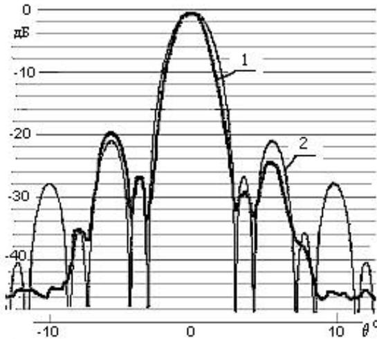
**Fig.3.** The pump antenna's (see Fig.1) directivity diagrams : 1- experimental; 2- theoretical.
