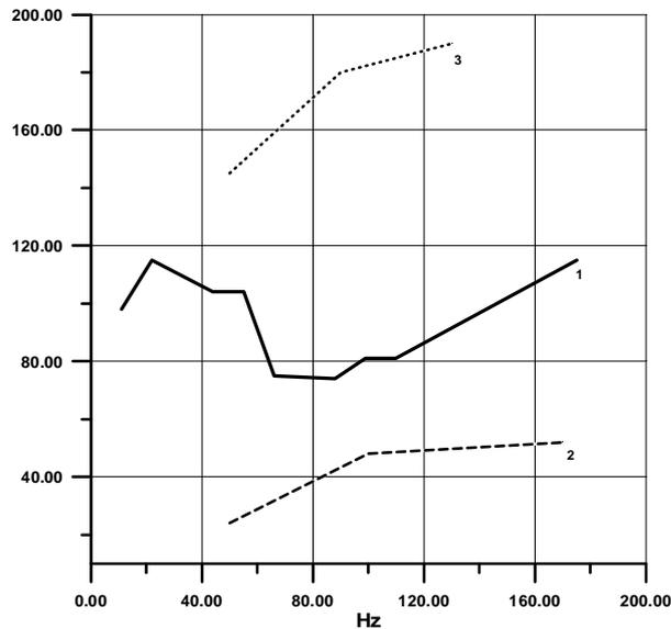
**Fig.3.** Frequency dependence of the transmission losses coefficient  $a(f)$  on the 200-km route (curve 1) in comparison with data [2].
