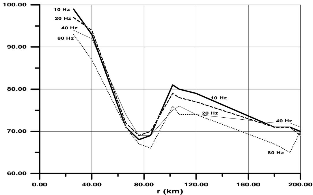
**Fig.1.** The results of a received signal intensity (in dB) measurements along the 200- kms route on the four frequencies.
